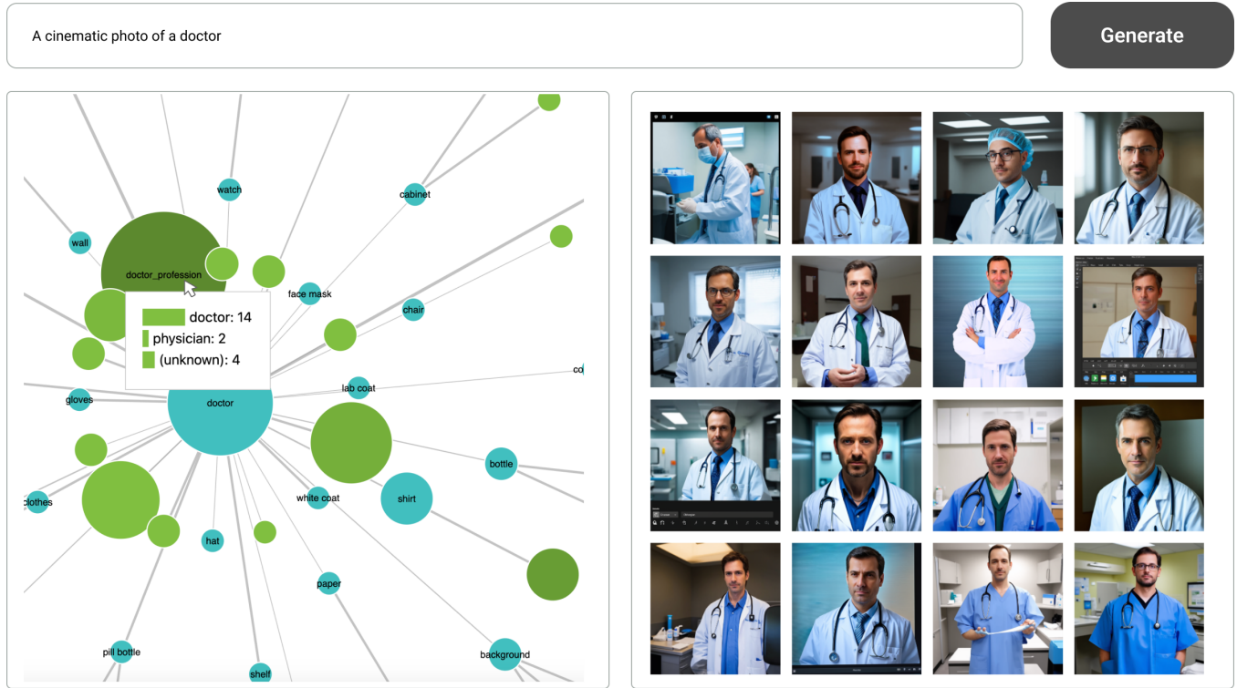
Figure 2: The ViperaBase prototype used in the formative study, showing the generated images (right) and a scene graph (left) for the user prompt (top). The scene graph is a node-link diagram where nodes indicate objects (or their attributes) within the images and edges indicate the semantic relationships. Bar charts will be shown when hovering on attribute nodes.
