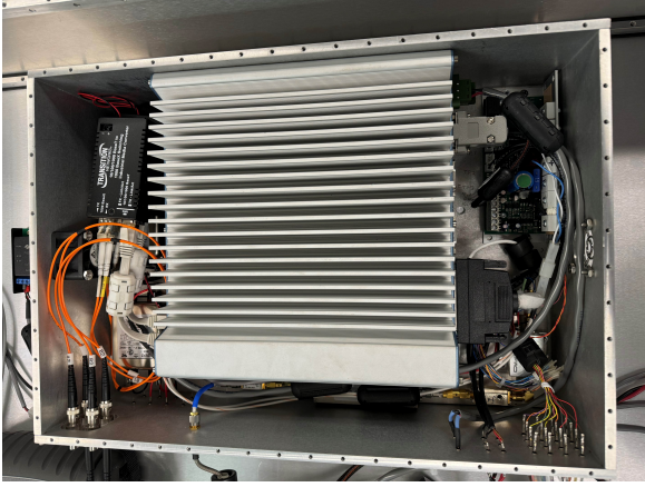
Figure 7. The shielded backend electronics box inside of EDGES-3, with the Nuvo computer inside. The various MezIO control wires can be seen exiting the box in the lower right, and the optical fiber leaves the box in the lower left, coming from the media converter visible in the upper left corner of the box.
