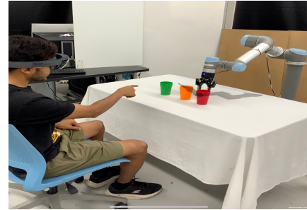
Fig. 1: Scenario that motivates the need for constant foreshadowing of the robot’s behavior. In ASD, this is achieved by using virtual shadows to continuously project the robot’s future state to assist in maintaining safer interaction.
