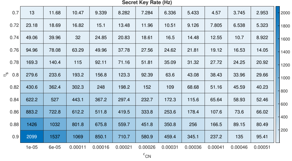
FIG. 12. (a) Simulated secret key rates for communication distance of 1000km with CNOT gate error rates ranging from 10^{-5} to 5.1 \times 10^{-4} and single photon source efficiency between 0.7 and 0.9, n_m = 100 .
