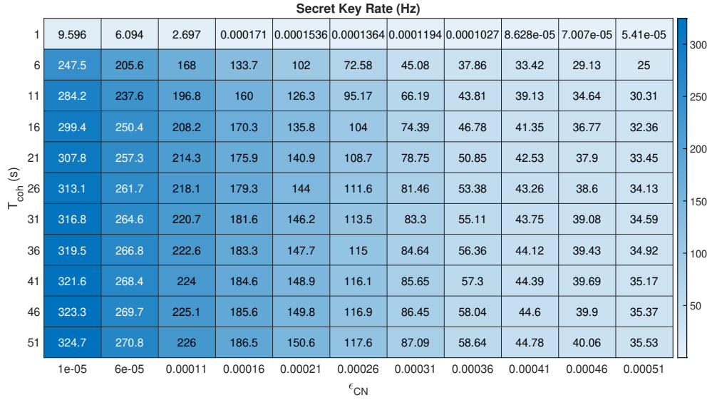
FIG. 13. Simulated secret key rates for communication distance of 1000km with CNOT gate error rates ranging from 10^{-5} to 5.1 \times 10^{-4} and coherence time of the qubit between 1s and 51s, n_m = 100 .
