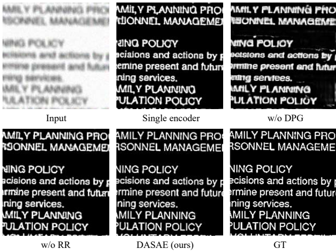
Fig. 13. Visual comparison of ablation results for DASAE. The visualizations correspond to the ablation settings listed in Table XI. Utilizing a single encoder maps all degradation types into an entangled space. Furthermore, the absence of either DPG or routing regularization hinders the extraction of accurate degradation representations with blurry artifacts. In contrast, DASAE restores images with sharp structures.
