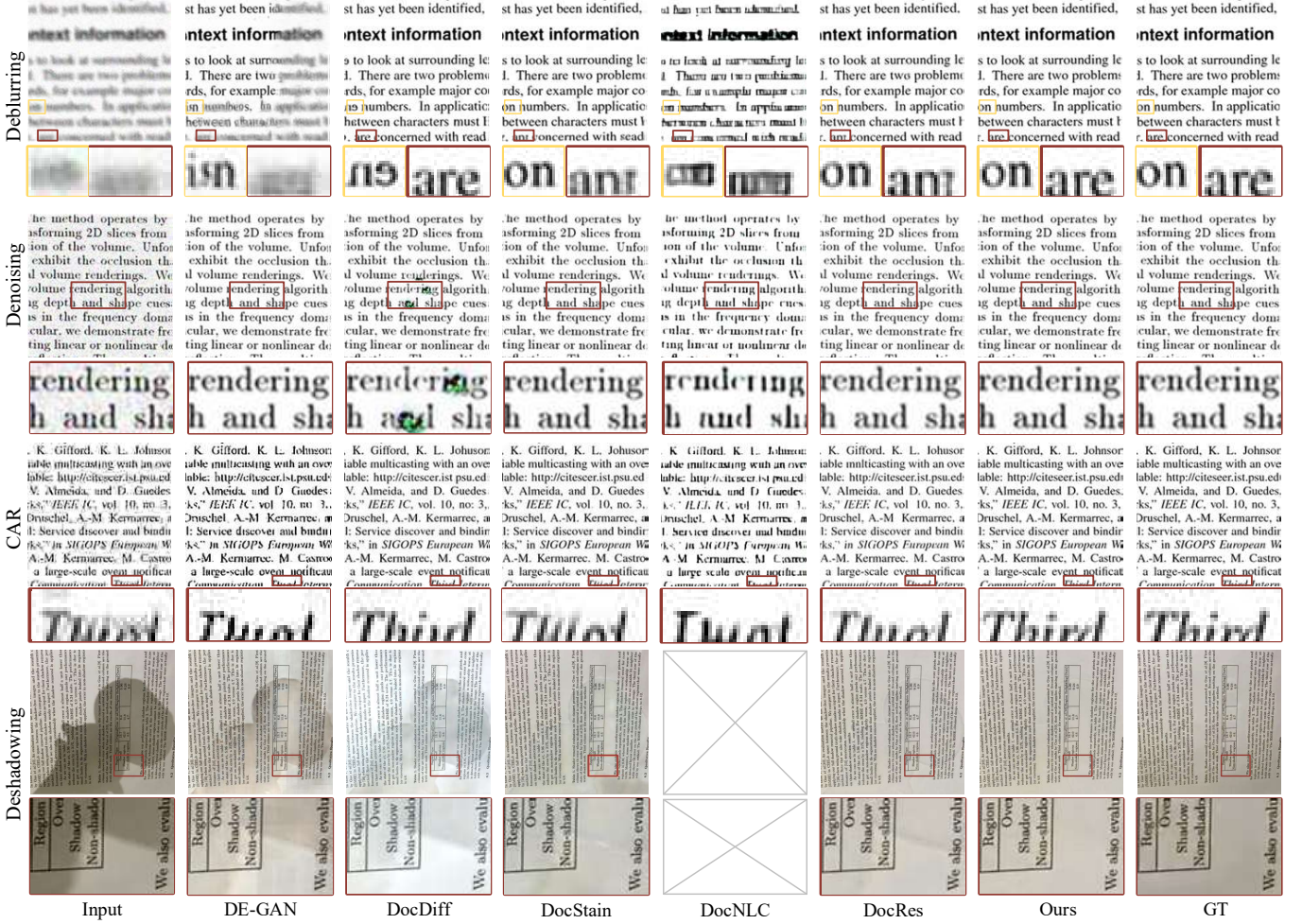
Fig. 6. Qualitative comparison across four restoration tasks: deblurring, denoising, CAR, and deshadowing, evaluated on the TDD, TDD_{CAR} , TDD_{noise} , and RDD datasets, respectively. As evidenced by the results on TDD and TDD_{CAR} , our method recovers clearer text boundaries and rectifies distorted strokes. This enhanced structural fidelity is consistent with the role of the DASAE, which predicts structure maps and injects high-frequency priors to guide the reconstruction. For denoising on TDD_{noise} and deshadowing on RDD, DocPure achieves clean background separation while preserving intricate details.
