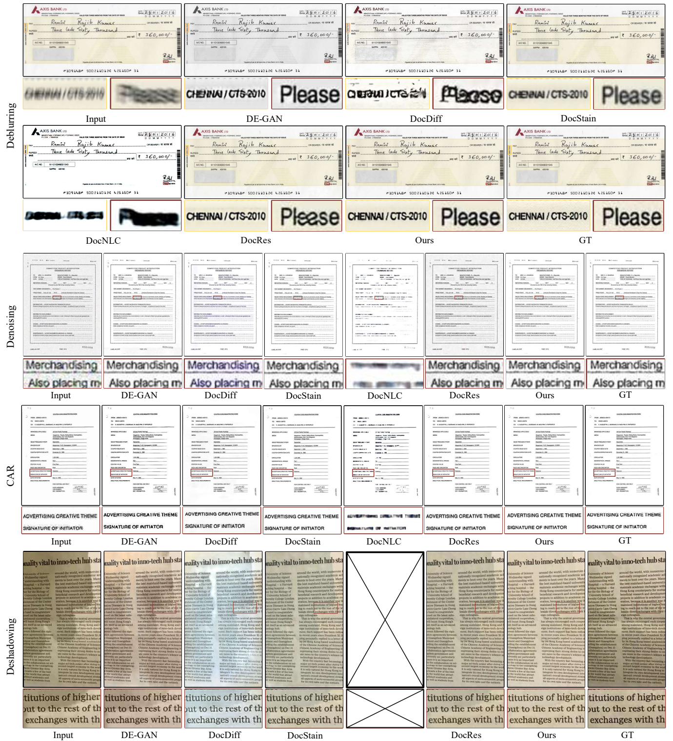
Fig. 15. Qualitative comparison of generalization capabilities across four image restoration tasks: deblurring, denoising, compression artifact reduction (CAR), and deshadowing, evaluated on the \text{BCSD}_{\text{blur}} , \text{FUNSD}_{\text{noise}} , \text{FUNSD}_{\text{CAR}} , and \text{OSR} datasets, respectively. The evaluation is conducted on document images with styles distinct from the training set. Leveraging our degradation-aware structure-guided wavelet modulation, our DocPure exhibits enhanced generalization to text patterns and complex backgrounds.
