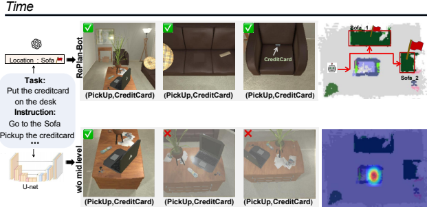
Figure 6. Comparison between RePlan-Bot with and without mid-level searching. The top row shows correct actions guided by commonsense-guided search mechanism, while the bottom row shows failed actions based on U-net.
