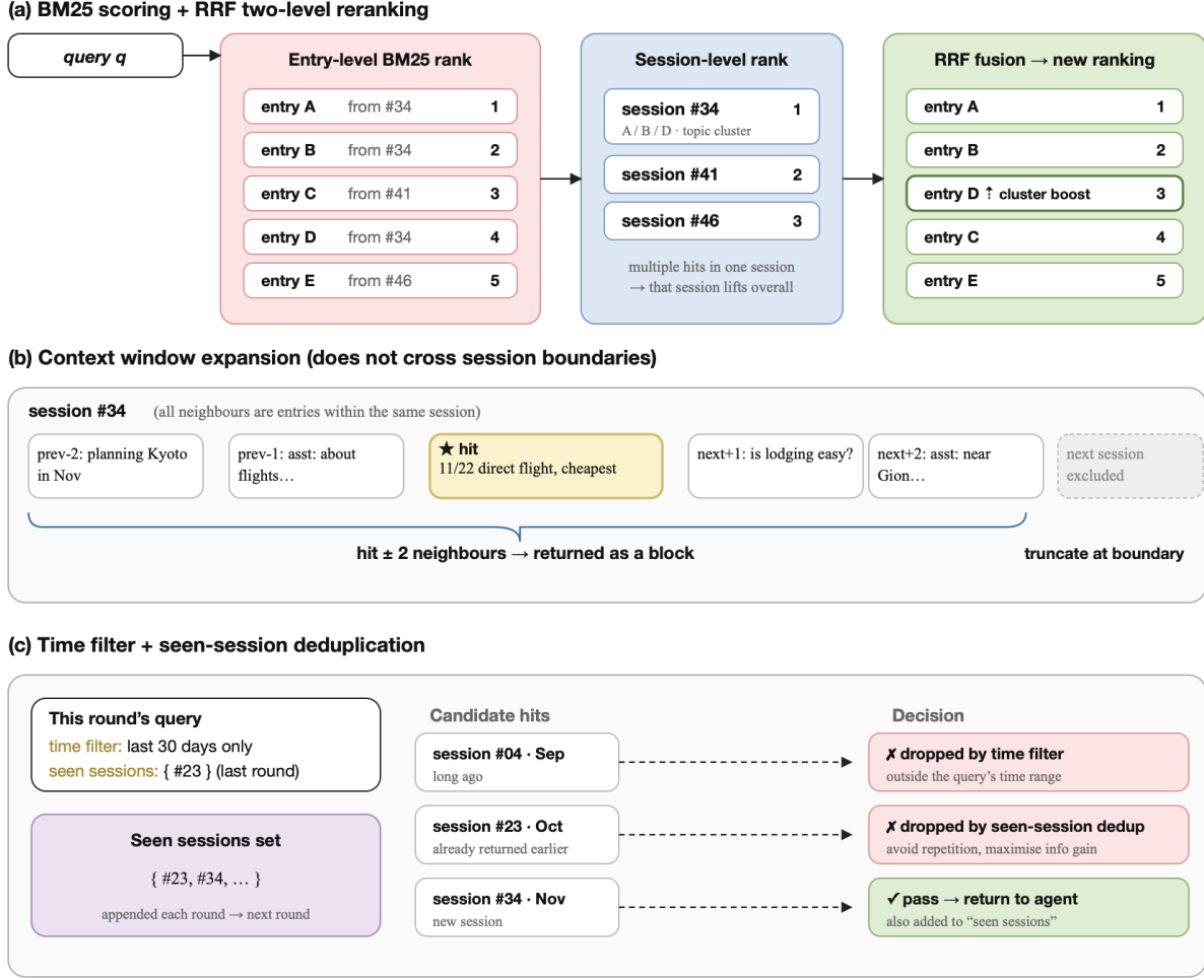
Figure 1 Search engine core mechanisms. (a) BM25 scoring with RRF two-level reranking: turn-level BM25 ranks (shown as entries ) are fused with session-level aggregate ranks via Reciprocal Rank Fusion—multiple hits within the same session boost that session’s entries. (b) Context window expansion: the matched entry plus \pm 2 neighboring turns are returned as a block, truncated at session boundaries. (c) Temporal filtering and seen-session deduplication: candidates outside the time range or from previously returned sessions are dropped, maximizing information gain per iteration.
