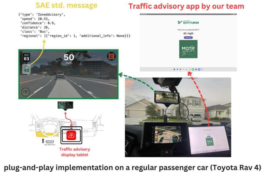
Figure 9: Illustrative advisory-speed application on a Toyota RAV4. The prototype demonstrates information delivery and display; safety-critical control and independent SAE-message conformance are outside the scope of this example.
