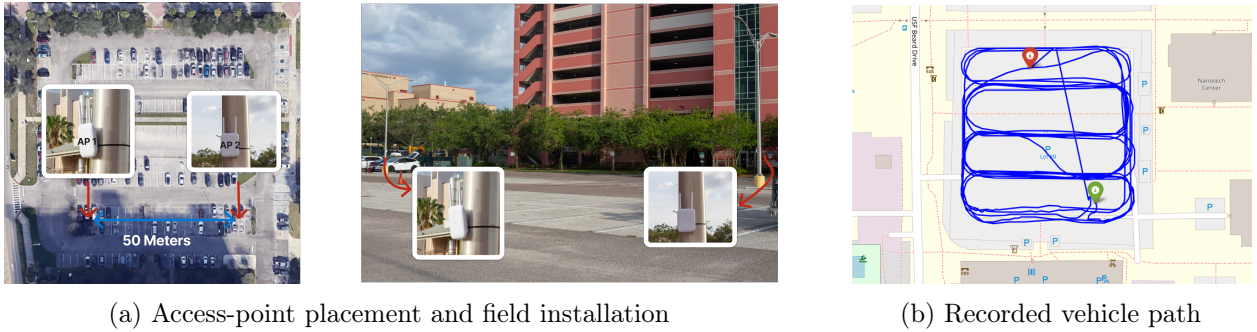
Figure 5: Moving-vehicle Wi-Fi experiment. The two access points were separated by 50 m; the vehicle completed repeated loops through the surrounding parking lot.
