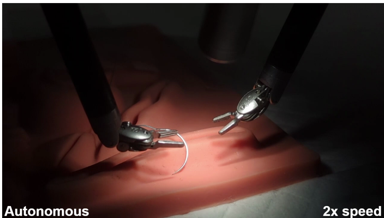
Movie S1: Successful end-to-end suturing rollout by GR00T-H on the SutureBot benchmark. GR00T-H controls the dVRK-Si to pick up and hand over the needle, perform needle throw and extraction, and complete the task with a knot tie.
