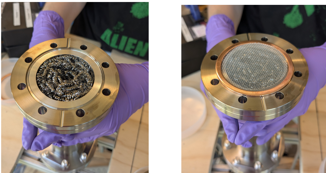
Figure 3: Stainless steel diffuser (left) and mesh (right) were installed at the purifier entrance, where LAr flows into the MS column.
