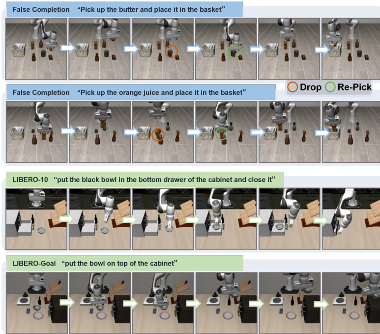
Fig. 6: Additional qualitative results in simulation on the False-Completion Benchmark, LIBERO-10, and LIBERO-Goal. In the False-Completion Benchmark, ReViP detects the object drop during execution and re-grasps the target, achieving true completion instead of prematurely terminating. On LIBERO-10 and LIBERO-Goal, ReViP consistently completes long-horizon tasks under diverse disturbances, environments, and object configurations. These visualizations highlight the complexity of the tasks and further demonstrate ReViP’s robustness, generalization, and execution capabilities.
