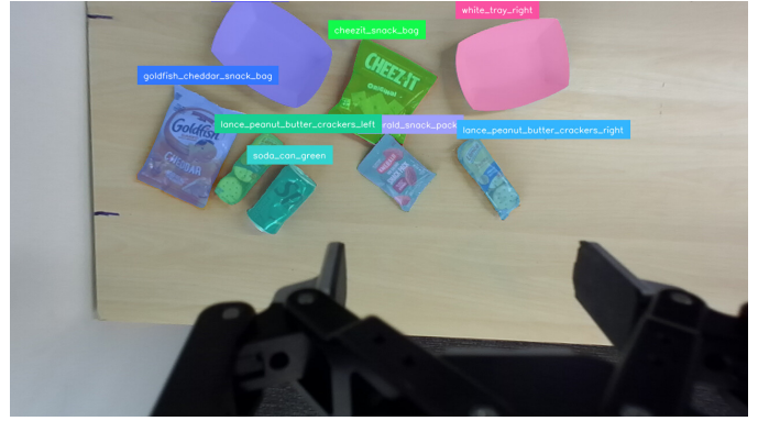
Fig. 7: Object Segmentation. SAM-2 generates eight pixel-level segmentation masks from the bounding boxes in Fig. 3c.
