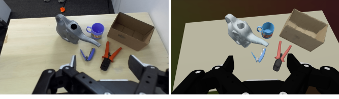
Fig. 4: Shape-Completion Mode. From the observed scene (left), RecGen [75] faithfully recovers the full geometry of each object (right), including the elephant watering can.
