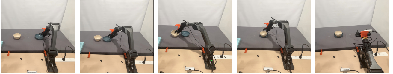
(a) Approach and grasp plate (b) Place plate on center (c) Approach and grasp bowl (d) Place bowl on plate (e) Return to home position
